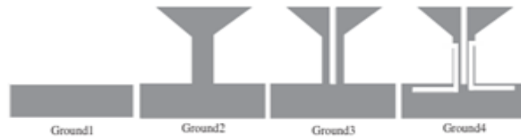
Figure 3. Progression steps for the bottom plane structure
