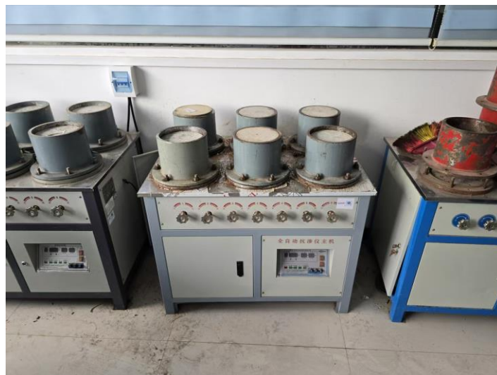
Figure 2 Concrete Permeability Resistance Test
