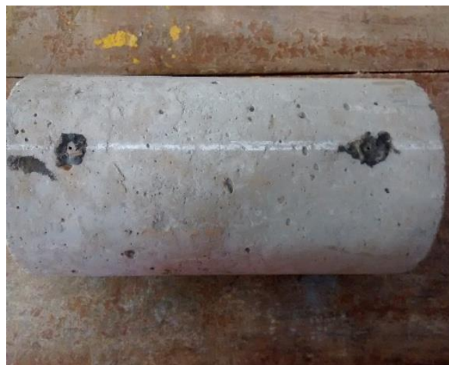
Figure 7 Set up for measuring drying shrinkage
