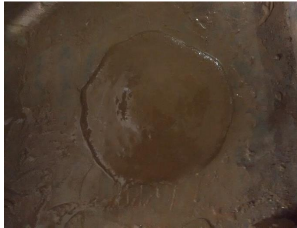
Figure 4 Mortar flow measurement using slump cone test (SCC-1)
