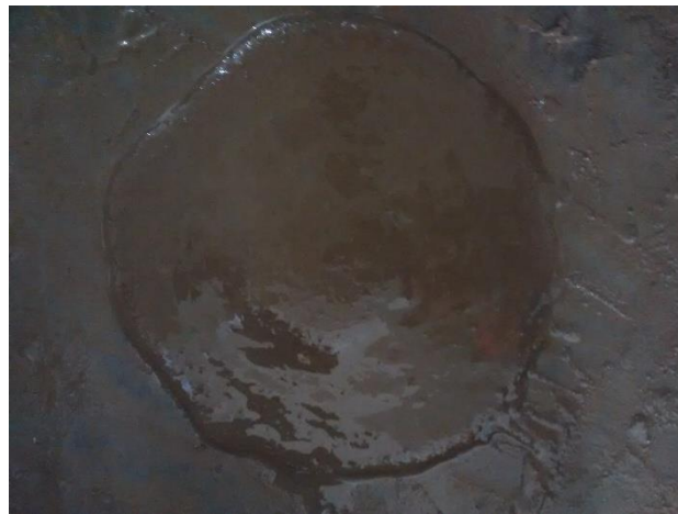
Figure 5 Mortar flow measurement using slump cone test (SCC-2)
