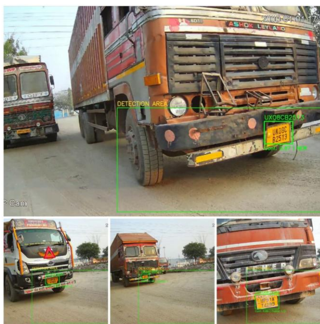
Figure 8: Real-time detection results demonstrating system performance across various environmental conditions and vehicle types
