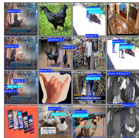
Fig. 18: Model predictions for batch 0. High overlap for person; incomplete detection for weapon.
