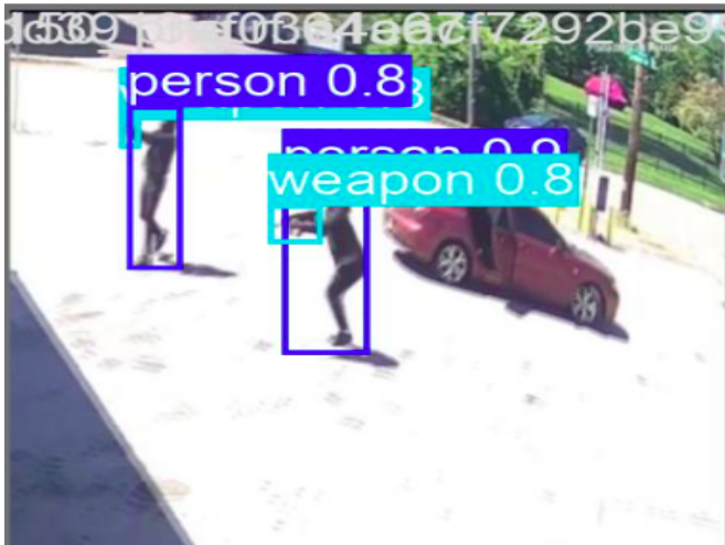
Fig. 10: Detection result — Two persons detected with confidence 0.8, and a weapon detected with confidence 0.8.
