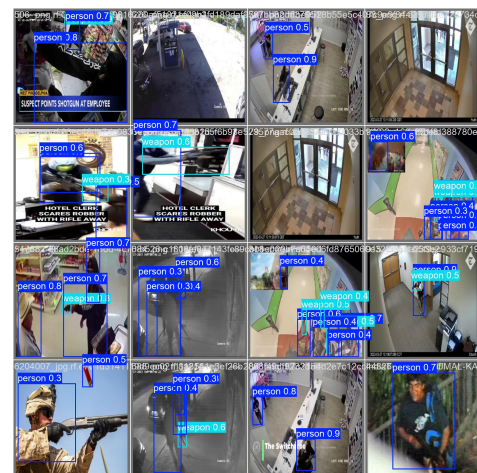
Fig. 22: Model predictions for batch 2. Person class well captured; weapon class often missed or confused with background.
