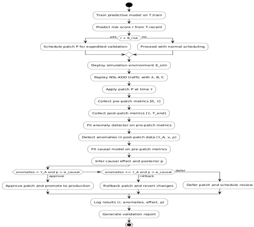
Fig. II. Autonomous Patch Validation Pseudo-Code Flow
