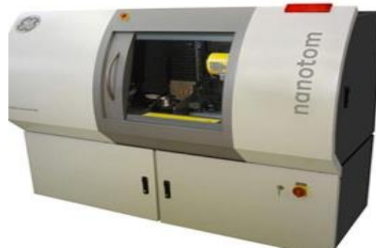
Figure 1. Phoenix Nanotom S Micro-CT Scanner Setup
