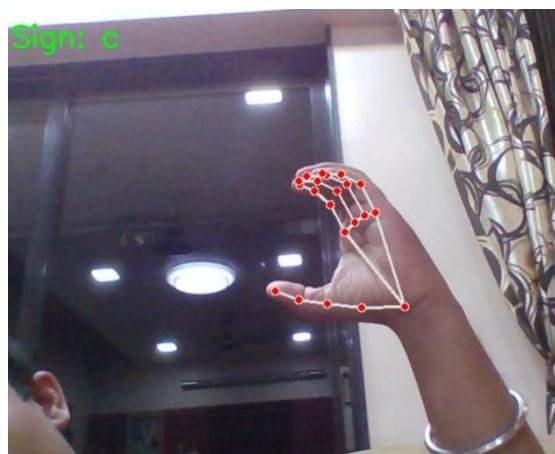
Figure 4: Real-time ASL prediction using the trained model. The system detects hand landmarks and predicts the corresponding sign
