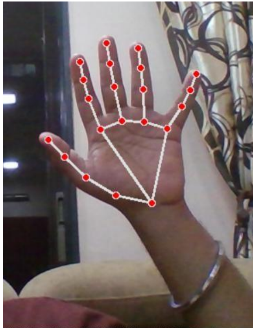
Figure 2: Hand landmark detection using MediaPipe. The X and Y coordinates of the fingertips (landmark IDs: 4, 8, 12, 16, and 20) were extracted as model inputs. These fingertip landmarks together formed a 10-dimensional feature vector for classification.
