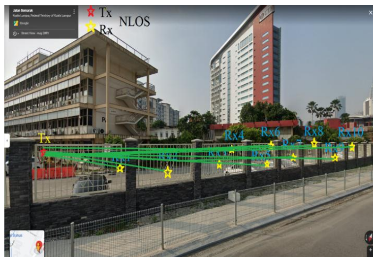
Figure 2. The measurement environment for the NLOS scenario
