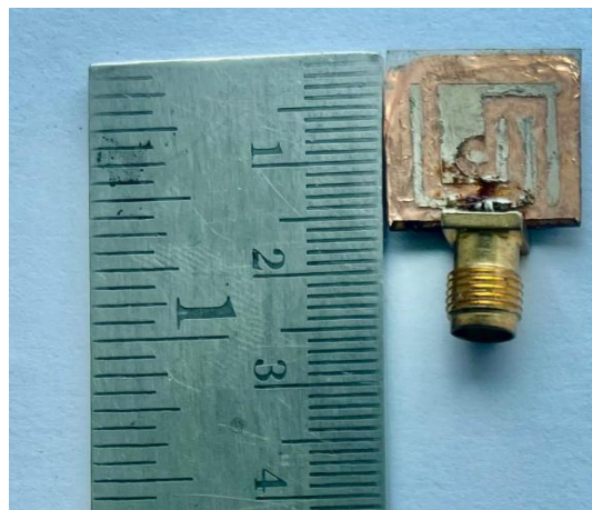
Figure 12: Fabrication of the proposed antenna
