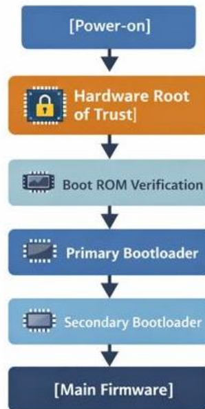
Figure 2. Multi-stage Secure Boot Process in Automotive ECU
