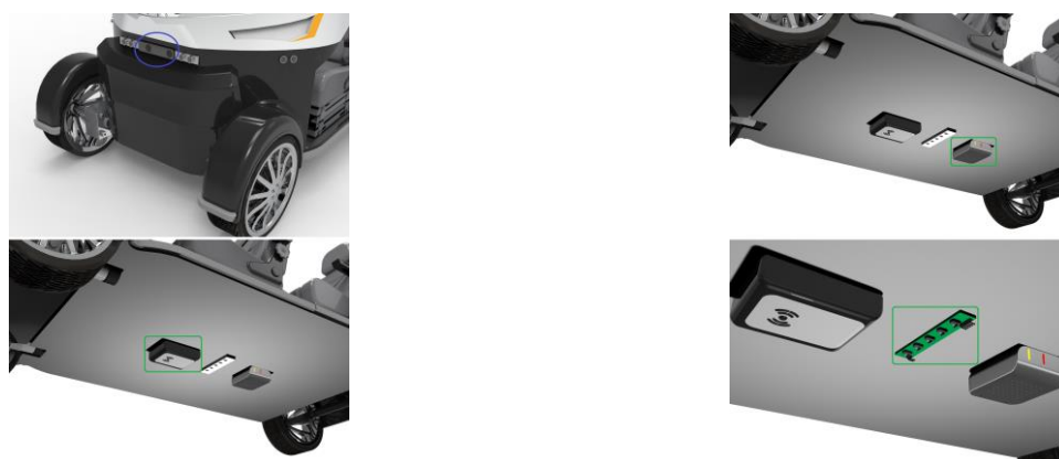
Fig. 2: Hetrogeneous Sensor Array: Left to Right; 1- Stereo Vision Camera, 2- RFID Transponders, 3- Bluetooth / Transponder , 4- Line Following Sensor Array
