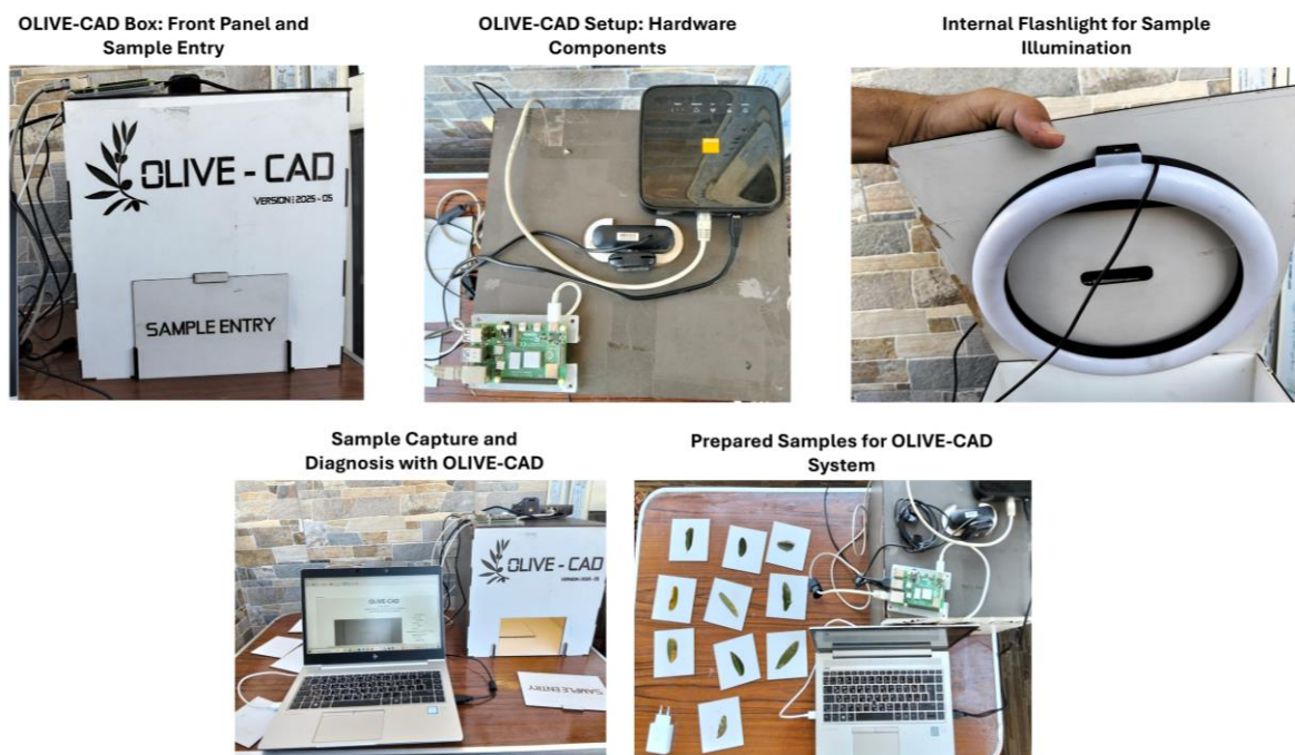
Figure 9. Detailed View of the OLIVE-CAD Diagnostic Box, Including Hardware Components, Internal Illumination, Operational Setup, and Prepared Sample Images
