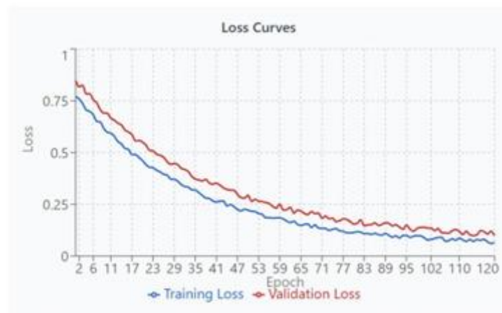
Figure 5: Training and Validation Loss Curve; Audio Model: GRU + Self-Attention Network (120 Epochs)
