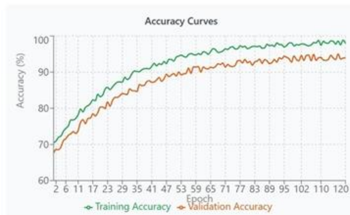
Figure 6: Training and Validation Accuracy Curve; Audio Model: GRU + Self-Attention Network (120 Epochs)
