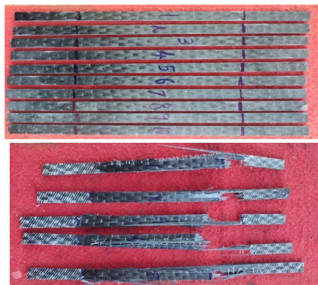
Figure 10: Tensile specimens before and after failure.
