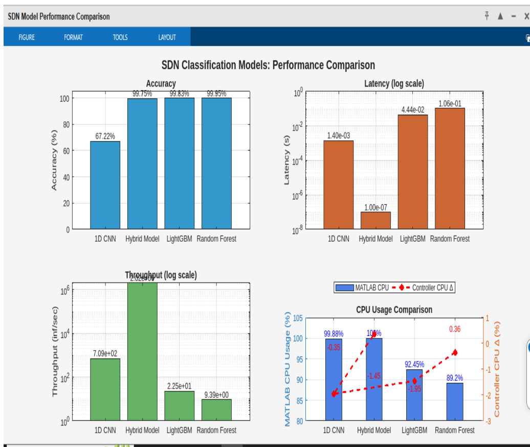
Figure 8. Performance comparison of SDN classification models across key metrics. This composite figure contains four subplots: (a) Accuracy (%), (b) Log-scale latency (s), (c) Log-scale throughput (inf/sec), and (d) CPU usage (blue bars for local CPU, red line for controller CPU delta). The data here reiterate earlier points: (a) all models except CNN achieve ~99% accuracy; (b) the Hybrid’s latency is orders of magnitude lower than others (visible as essentially 0 on log-scale, vs. CNN at 1e-3, LightGBM at 4e-2, RF at 1e-1 seconds); (c) correspondingly, Hybrid’s
