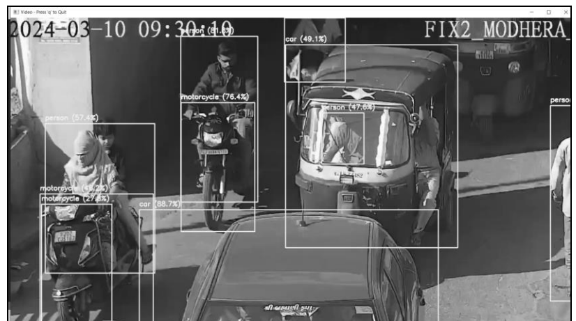
Fig. 4. Vehicle Recognition, Categorisation and number plate detection from a Dataset of Mehsana Traffic Videos
