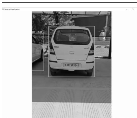
Fig. 3. Vehicle Recognition, Categorisation and number plate detection from a Dataset of SPU Parking Videos
